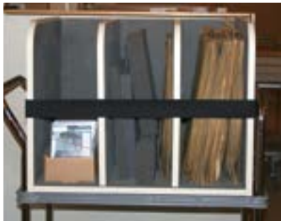
Metal cart with Library of Congress designed "topper." A Velcro strap provides added protection in case items roll or slip.
