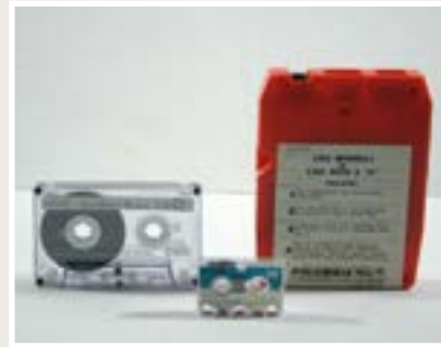
Comparison of compact cassette, microcassette, and 8-track cartridge
