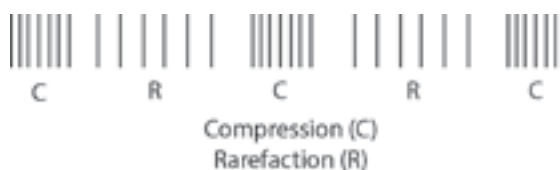
Fig. 1.1: An example of compression and rarefaction
